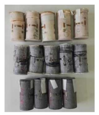
Fig. 2. Photographs of failed specimens after the direct tensile and uniaxial compressive tests. a – After direct tensile test, b – After uniaxial compressive test
